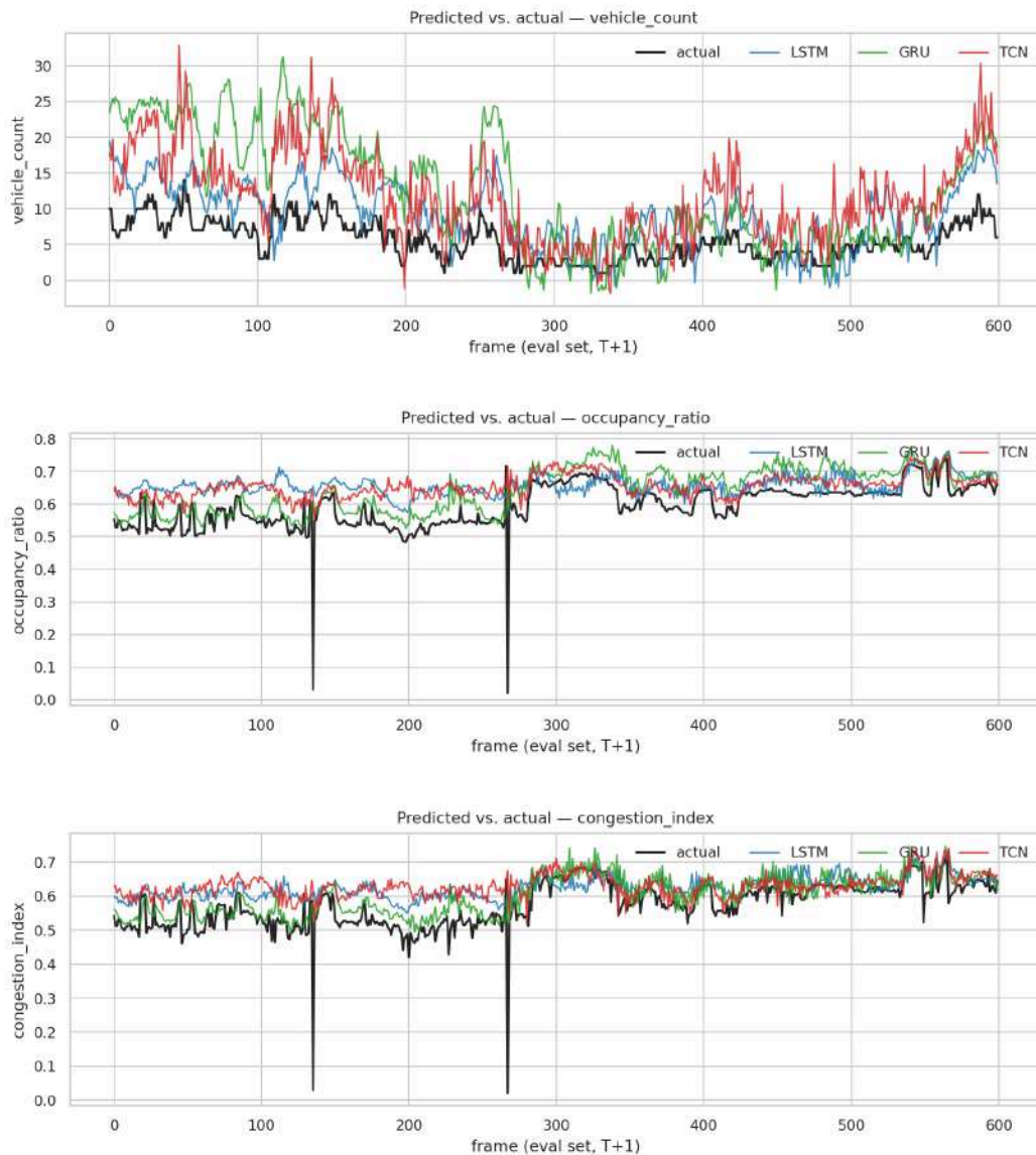
Figure 18: Predicted vs. actual time series for vehicle_count (top), occupancy_ratio (middle), and congestion_index (bottom) on the held-out YOLOv5l evaluation stream. All three estimators are overlaid against the ground truth.
